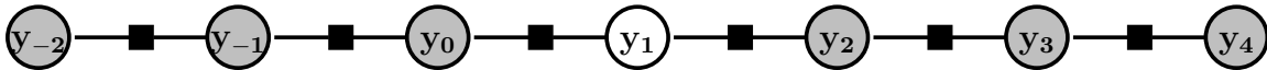
Figure 4-3: Factor graph for the interpolation problem in Figure 4-2. The circle nodes represent the random variables and the solid squares represent the derivative statistics constraint. Here, the shaded nodes indicate observed values.
