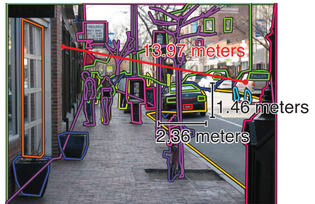
Fig. 13. Snapshot of the 3D measuring tool. Once we compute the 3D coordinates for a depicted scene, we can make measurements of scene components. Here, we show the height and width of the car, which is 13.68 meters away from the camera center. We can also compute the distance between any two points in the scene, such as the selected points on the building and the truck.
